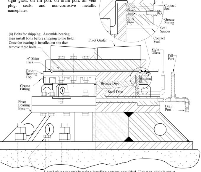
Level pivot assembly using leveling screws provided. Use non-shrink grout under pivot assembly. Back off leveling screws.
