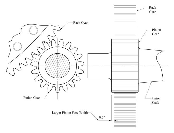
Figure 6.8.1.2.3-1—Typical Pinion and Ring Gear Assembly on a Bascule Bridge
