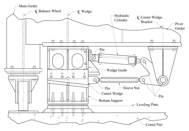
Figure 6.8.2.5-2—Typical Center Wedge Assembly
