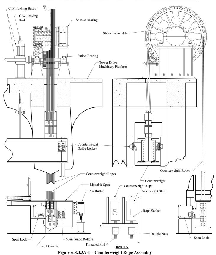
The above figure shows the design for equal rope lengths. The figure was taken from the Prospect Bridge contract drawings, LADOTD 2009, State Project 065-91-0016.
