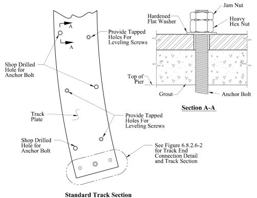
Figure 6.8.2.6-3—Standard Balance Wheel Track Example
