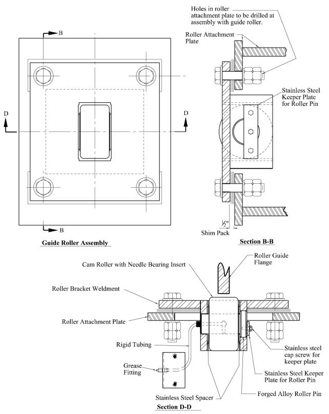
Figure 6.8.3.8-2—Example of a Vertical Lift Bridge Guide Roller Assembly For the Free End
