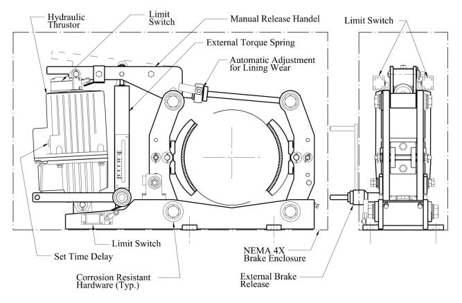
Figure 6.7.13.2-1—Thruster Type Electrically Released Shoe Brake
