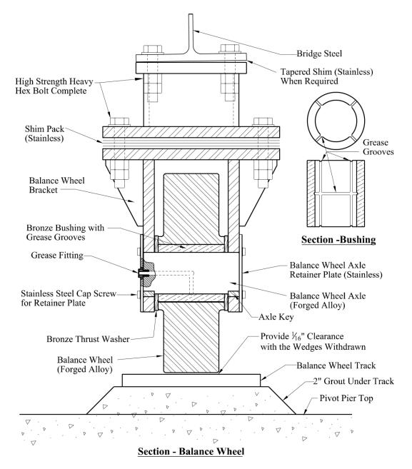
Figure 6.8.2.6-1—Typical Balance Wheel Assembly
