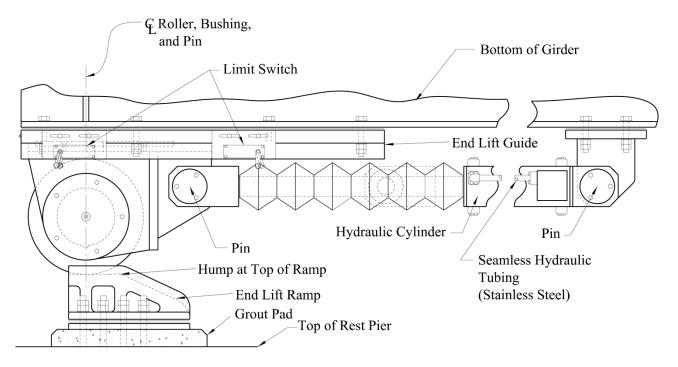
Figure 6.8.2.4-1—Typical Hydraulic End Lift Assembly
