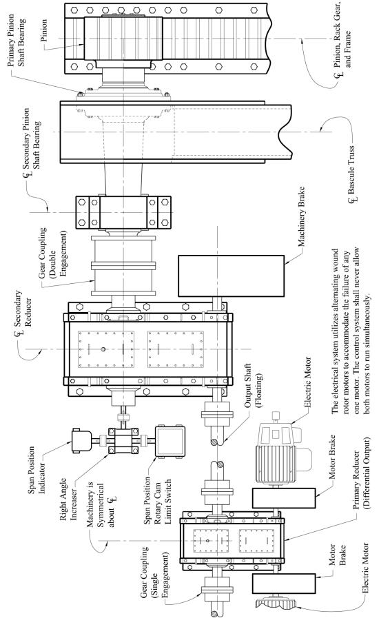
Figure 6.8.1.1-1 — Span Drive Machinery Layout for a Rolling Lift Bascule Bridge
